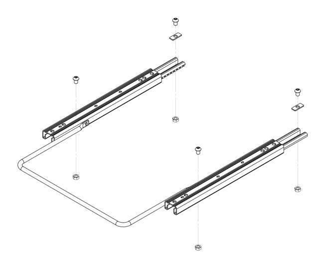
**Step 1**Remove bolts from seat base and place these to one side as you will require these later.
