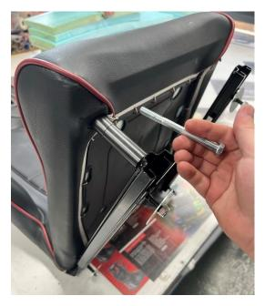
Slide runner handle onto the runner clips as shown in image 7 and 8
