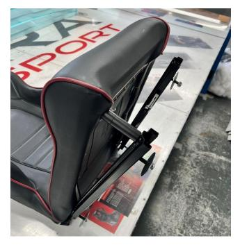
Insert the long hex head bolt through the runner and spacer and tighten as shown as in image 6
