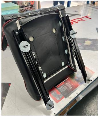
Flip seat over to face up and slide runners back to allow access to front bolt holes. Insert spacers in the gap as shown in image 5
