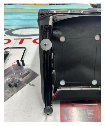
Use cap head bolt to fix runner to seat at rear bolt hole as shown in image 3
