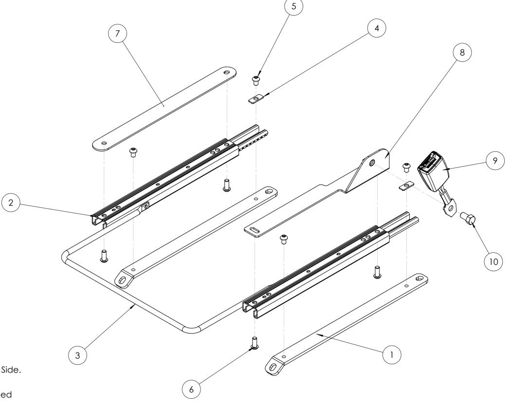
NOTE: This drawing is configured for UK Driver's Side. For UK Passenger Side, the Spacer Bar and the Seatbelt Brackets must be on opposite sides in relation to this drawing. Therefore, a Left-Handed Seatbelt Bracket will be required.
