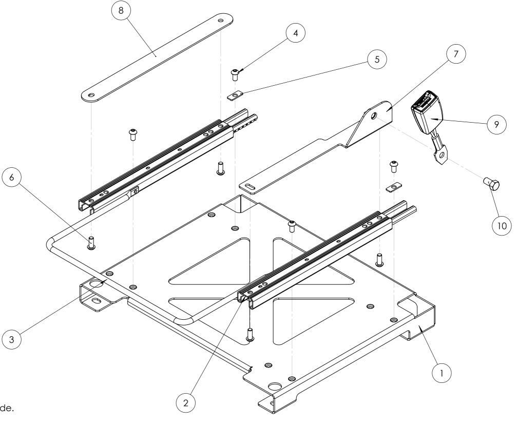
NOTE: This drawing is configured for UK Driver's Side. For UK Passenger Side, the Spacer Bar and the Seatbelt Brackets must be on opposite sides in relation to this drawing. Therefore, a Left-Handed Seatbelt Bracket will be required.
