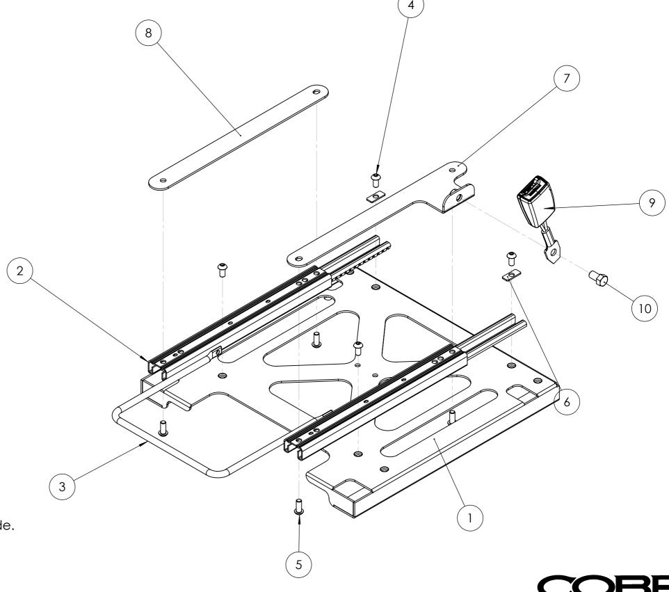
NOTE; This drawing is configured for UK Drivers side. For UK passenger side, the spacer bar and the seatbelt bracket must be on opposite sides in relation to this drawing. therefore, a left handed seatbelt bracket will be required.
