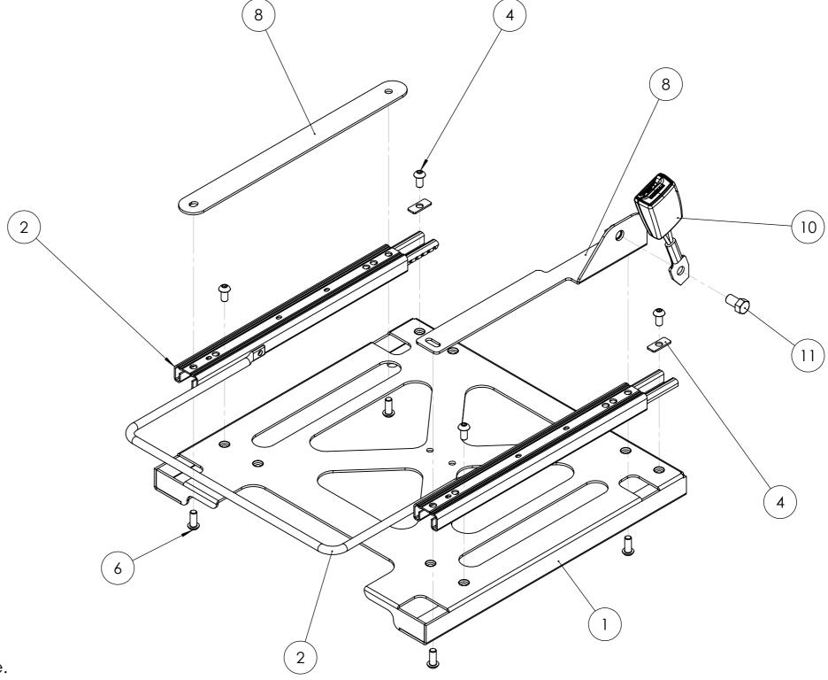
NOTE; This drawing is configured for UK Drivers side. For UK passenger side, the spacer bar and the seatbelt bracket must be on opposite sides in relation to this drawing. therefore, a left handed seatbelt bracket will be required.
