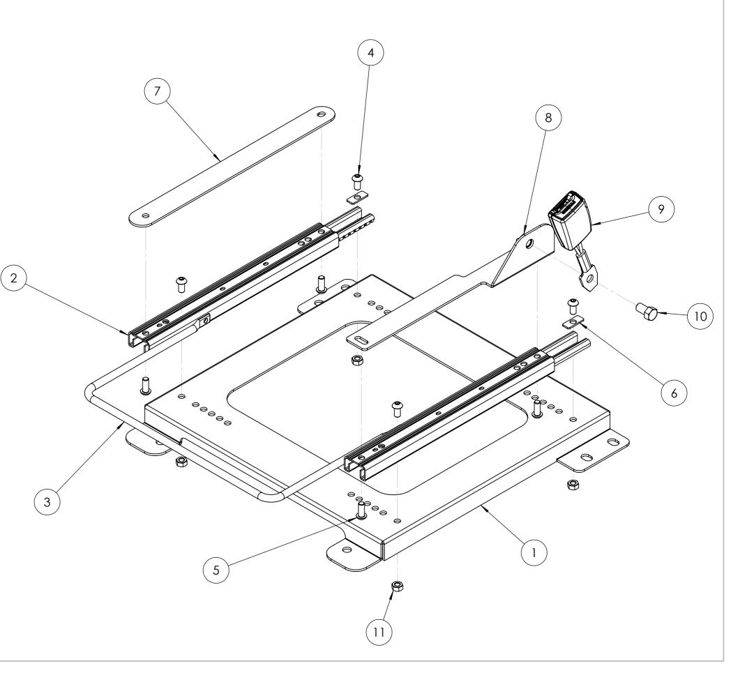
NOTE: This drawing is configured for UK Driver's Side. For UK Passenger Side, the Spacer Bar and the Seatbelt Brackets must be on opposite sides in relation to this drawing. Therefore, a Left-Handed Seatbelt Bracket will be required.
