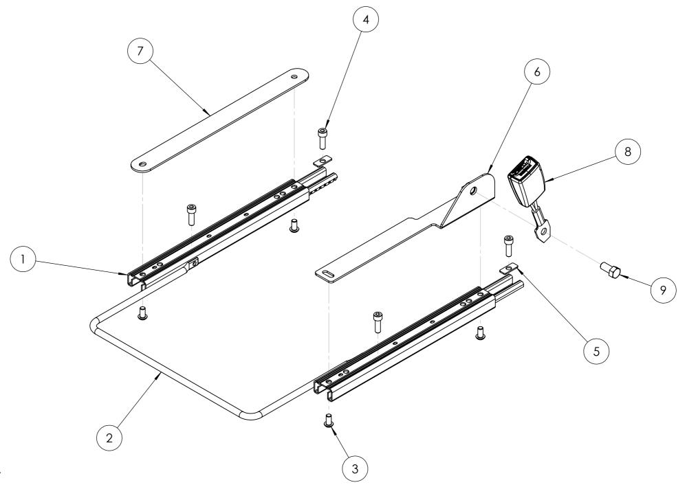
NOTE: This drawing is configured for UK Driver's Side. For UK Passenger Side, the Spacer Bar and the Seatbelt Brackets must be on opposite sides in relation to this drawing. Therefore, a Left-Handed Seatbelt Bracket will be required.
