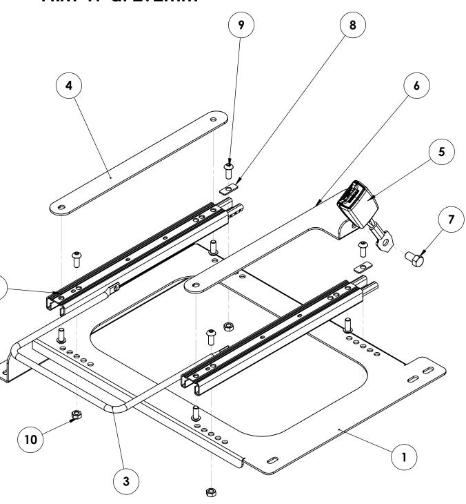
NOTE: This drawing is configured for UK drivers side. For UK passenger side, the spacer bar and the seatbelt brackets must be on opposite sides in relation to this drawing. Therefore, a left handed seatbelt bracket will be required.
