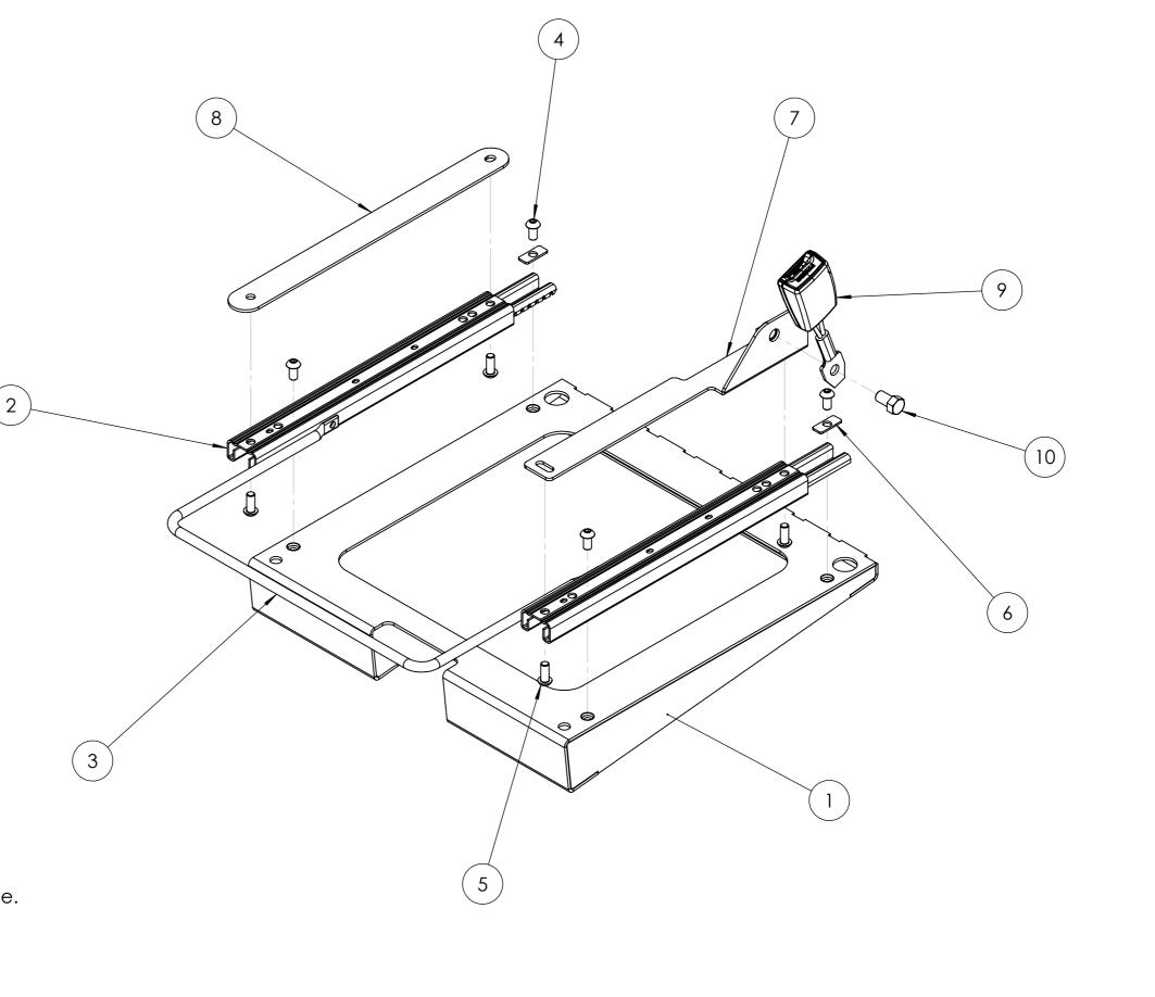
NOTE: This drawing is configured for UK Driver's Side. For UK Passenger Side, the Spacer Bar and the Seatbelt Brackets must be on opposite sides in relation to this drawing. Therefore, a Left-Handed Seatbelt Bracket will be required.
