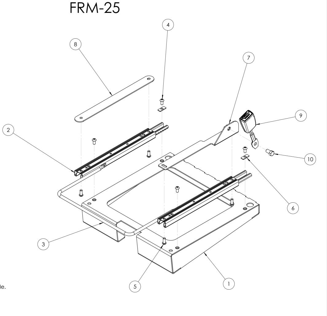
NOTE: This drawing is configured for UK Driver's Side. For UK Passenger Side, the Spacer Bar and the Seatbelt Brackets must be on opposite sides in relation to this drawing. Therefore, a Left-Handed Seatbelt Bracket will be required.
