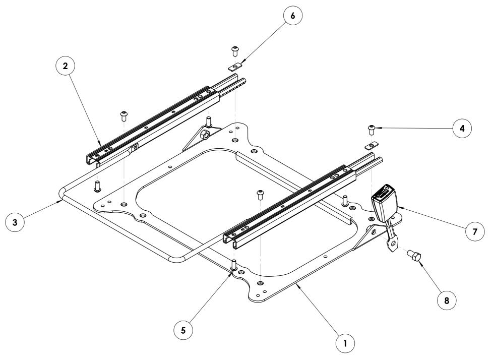
NOTE: This drawing is configured for UK Driver's Side. For Passenger Side, the seatbelt receiver must be attached to the opposing side of the frame in relation to this drawing. The seatbelt receiver used here is for illustrative puposes only, we recommend using the OE seatbelt receiver for this application.
