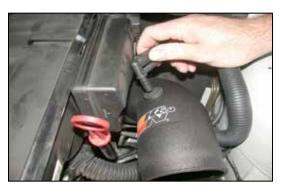
13. Insert the factory vent tube into the grommet in the intake tube as shown.
