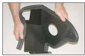
14. Install the provided edge trim onto the heat shield as shown.
