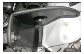
18. Reinstall the lower air box locator removed in step #10 and resecure the heater hose.
