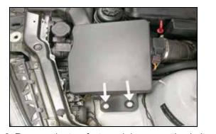
3. Remove the two factory air box mounting bolts
