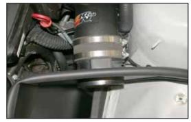
21. Install the mass air sensor assembly into the heat shield and onto the K&N $^{\mbox{\tiny \$}}$  intake tube, secure with the provided hose clamp.
