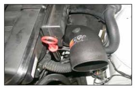
12. Install the intake tube into the factory lower intake tube and secure with the factory hose clamp.
