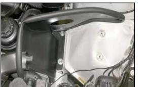
17. Install the heat shield assembly into the vehicle and secure with the provided fender washers and
