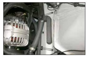
9. Unclip the rubber strap, which secures the heater hose to the lower air box locator.
