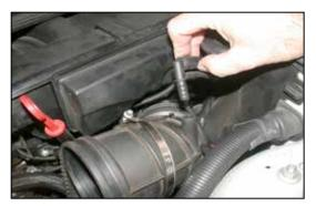
7. Pull up on the vent tube to dislodge it from the intake tube as shown.
