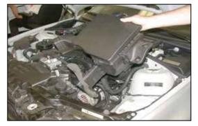
6. Lift the air box from the rear and remove it from the vehicle.
