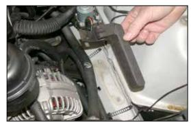
10. Pull up the lower air box locator to remove it from the mounting studs and then from the vehicle.
