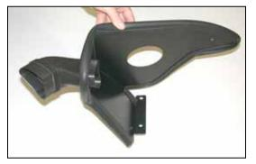
16. Install the fresh air duct into the heat shield as shown.
