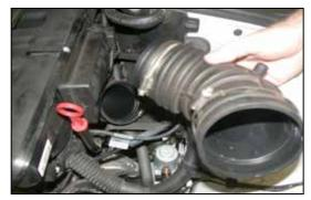
8. Loosen the lower hose clamp, which secures the upper intake tube to the lower intake tube, and then remove the upper intake tube from the vehicle.
