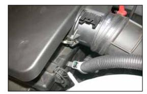
5. Unhook the wiring harness retainer shown from
