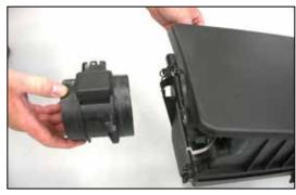
19. Unhook the two mass air sensor retaining clips and remove the mass air sensor from the air box.
