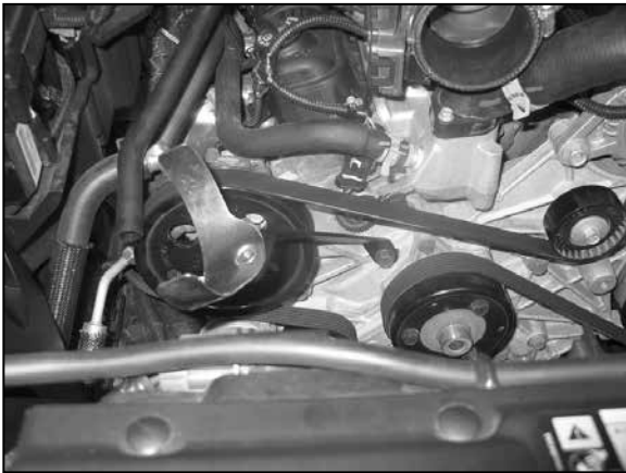
12. Install the tube mounting bracket assembly onto the engine and secure with the bolt removed in step #10. NOTE: Be sure the bracket sits flush to the engine.
