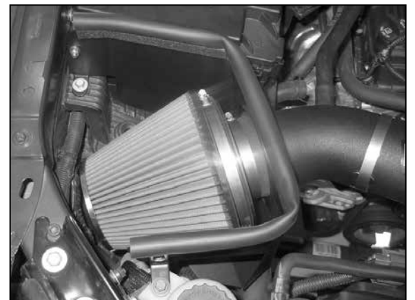
24. Install the K&N® air filter assembly on the intake tube and secure with the provided hose clamp as shown.
