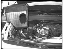
5. Pull up firmly on the air box assembly and remove it from the vehicle as shown.
