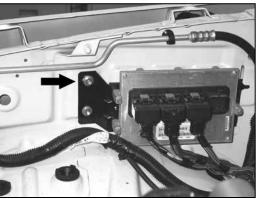
7. On 2007 model year vehicles, remove the ECU mounting nut shown.
