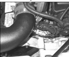
17. Re-connect the air temperature sensor electrical connection.
