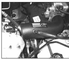
18. Connect the crank case vent hose to the 90° fitting installed into the K&N® intake tube as shown.
