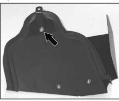
22. On 2007 model year vehicles, install the heat shield mounting bracket (#07805) to the side of the heat shield using the provided hardware.
