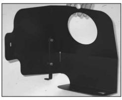
19. Install the heat shield mounting bracket (#07159) onto the heat shield using the provided hardware as shown.
