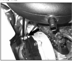
16. Secure the tube mounting bracket to the timing cover with the provided hardware as shown.
