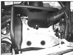
23. Install the heat shield into the engine compartment. Align the bottom rear mounting bracket with the threaded stud on the lower inner fender. Align the upper rear mounting bracket with the ECU mounting stud. Secure with the factory ECU mounting nut and provided hardware.
