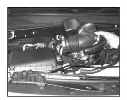
4. Loosen the two hose clamps that secure the stock intake tube, then remove the stock intake tube as shown.
