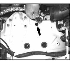
6. Remove the inner air box retaining grommet as shown.
