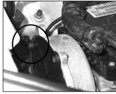
8. Remove the timing cover bolt (shown).
