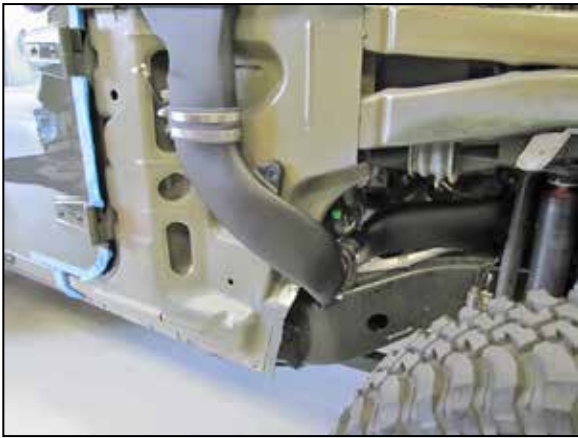
48. Install the provided coupler hose (08698) onto the corner tube, and then install the Corner tube assembly as shown, snug the hose clamps but leave them loose enough to provide adjustment.
