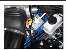
4. Disconnect the vacuum line from the stock intake tube as shown.
