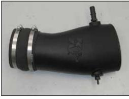
20. Install the provided silicone hose (08695) onto the K&N<sup>®</sup> intake tube, slide the hose all the way onto the K&N<sup>®</sup> intake tube; do not tighten at this time.
