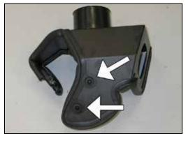
15. Install the factory mounting grommets to the two mounting posts installed on the K&N<sup>®</sup> heat shield assembly as shown.
