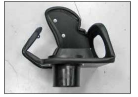
11. Install the mas air sensor into the heat shield, rotate the sensor 180° so the sensor boss is pointed downward, and then secure with the provided hardware.
