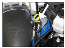
23. Connect the vent line to the 3/16" fitting installed into the K&N^ ${\ensuremath{\mathbb S}}$  intake tube.
