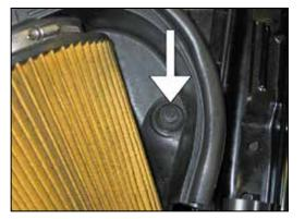
3. Remove the bolt that secures the airbox housing to the inner fender.
