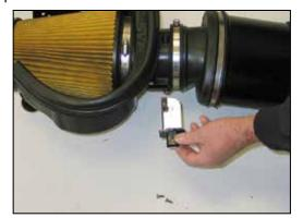
12. Remove the two screws securing the mass air sensor to the factory housing, then remove the mass air sensor as shown.
