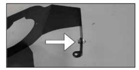
9. Install the heat shield mounting bracket (07158A) onto the heat shield using the provided hardware.
