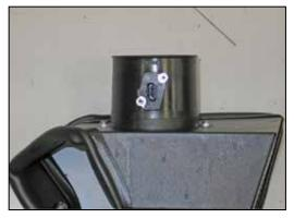
13. Install the mass air sensor into the K&N<sup>®</sup> mass air sensor housing and secure with provided hardware.
