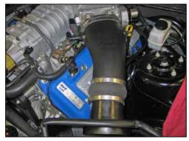
21. Install the K&N<sup>®</sup> intake tube into the silicone hose at the throttle body and align with the mass air sensor housing. Slide the silicone hose down the K&N<sup>®</sup> intake tube onto the mass air sensor housing. Align the tube for best fit and then secure with the provided hose clamps.
