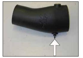
17. Install the provided 3/16" vacuum fitting into the K&N<sup>®</sup> intake tube as shown.
