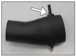
18. Install the quick disconnect fitting into the K&N<sup>®</sup> intake tube as shown.
