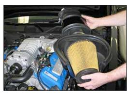
7. Disconnect the intake tube from the throttle body and then remove the complete intake system from the vehicle.
