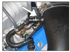
22. Connect the crankcase vent line to the quick disconnect fitting installed into the K&N<sup>®</sup> intake tube.
