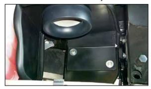
11. Using the provided hardware, secure the heat shield assembly to the nut-serts as shown. NOTE: finger tighten the bolts as some adjustment may be necessary.
