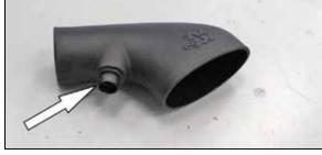
14. Install the provided grommet and quick disconnect fitting into the K&N<sup>®</sup> intake tube as shown.
