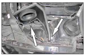
19. Secure the heat shield to the air filter housing studs with the provided hardware.
