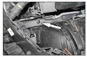
6. Remove the lower air filter mount from the frame rail.
