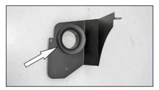
7. Install the filter adapter into the K&N $^{\odot}$  heat shield and secure with the provided hardware.
