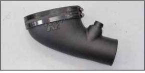
16. Install the provided coupling hose (08619) onto the K&N $^{\rm \tiny 6}$  intake tube and slide it as far as possible on.
