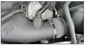
18. Connect the crank case vent hose to the quick disconnect fitting on the K&N<sup>®</sup> intake tube.
