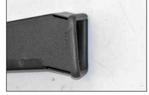
12. Install the small edge trim onto the K&N $^{\otimes}$  fresh air duct as shown.
