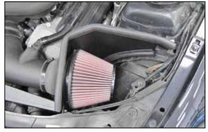
20. Install the K&N<sup>®</sup> air filter and secure with the provided hose clamp.
