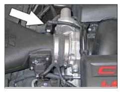
19. Install the K&N® intake assembly into the silicone hose on throttle body and onto the mounting studs. Secure with the provided hose clamp. Reconnect the crank case vent line.
