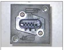
8. Install the mass air sensor into the K&N® mass air sensor adapter and secure with the provided screws.
