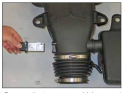
7. Remove the two screws which secure the mass air sensor to the stock intake tube and then remove the mass air sensor from the intake tube as shown.
