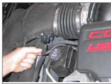
3. Disconnect the mass air sensor electrical connection as shown.
