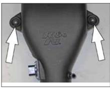
14. Install the two mounting grommets into the K&N® intake tube.
