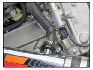
11. Install the crank case vent hose onto the fitting installed into the K&N® intake tube.
