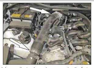
4. Loosen the two hose clamps securing the factory intake tube and then remove the factory intake hose from the vehicle.
