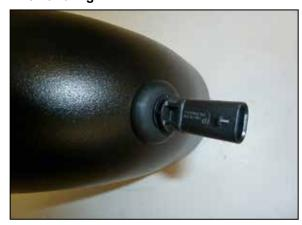
8. Install the provided grommet and factory temp sensor onto the K&N<sup>®</sup> intake tube.
