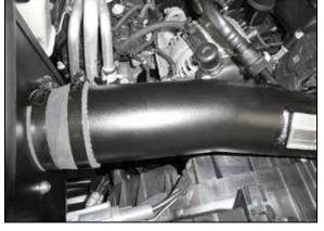
13. Connect the crank case vent line to the K&N<sup>®</sup> intake tube.
