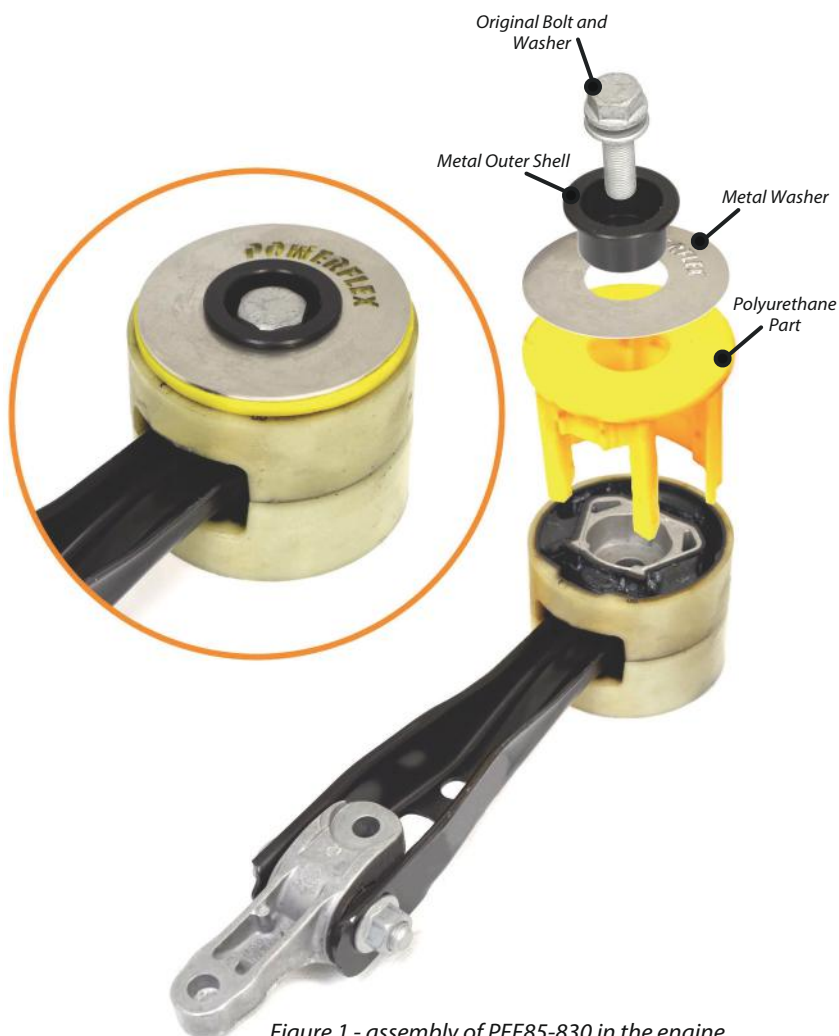
Figure 1 - assembly of PFF85-830 in the engine mount
