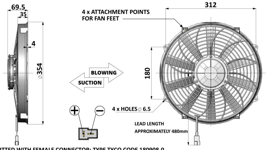
FAN FITTED WITH FEMALE CONNECTOR: TYPE TYCO CODE 180908-0
