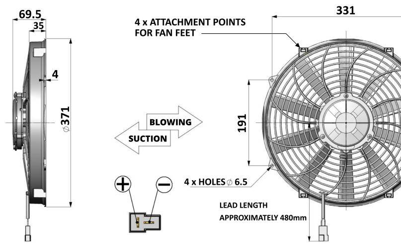
FAN FITTED WITH FEMALE CONNECTOR: TYPE TYCO CODE 180908-0 (MALE CONNECTOR: REVOTEC RTB-2)
