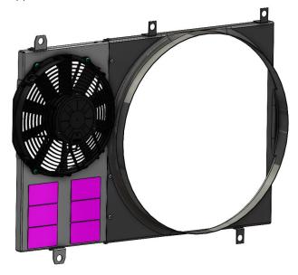
8. Refit the new assembly back into the vehicle and connect the new fan to the original fan wiring.
