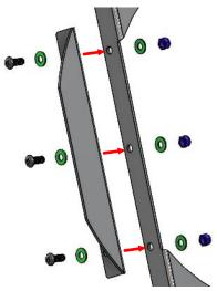
4. Attach the shroud mounting brackets to the top and bottom of shroud using the supplied M5 nuts, bolts and washers, there is the option for 1 or 2 upper mountings depending on the installation, the optional bracket is highlighted red below. There is a certain amount of built in adjustment in the brackets to allow for any imperfections in the original shroud mounts.
