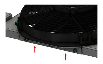
6. Using the supplied 5mm self drilling screws, with a suitable electric screw driver attached the shroud at the upper and lower mounting points (pre-drilled) then making sure the assembly is straight, use the remaining self-drilling screws to attached the remaining 3 mounting holes (not drilled).
