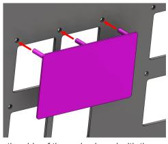
3. Loosley attach the side closure plate to the side of the main shroud with the supplied M5 nuts, bolts and washers.
