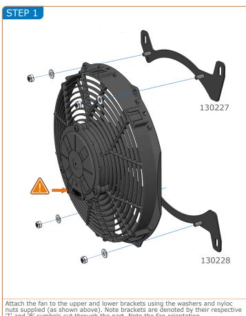
Attach the fan to the upper and lower brackets using the washers and nyloc nuts supplied (as shown above). Note brackets are denoted by their respective 'T' and 'B' symbols cut through the part. Note the fan orientation.
