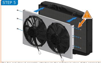
The fan and shroud assembly attaches to the radiator in place of the original fan shroud, using the existing side fixing points. Use the bolts saved from step 1 to secure the fan kit to the radiator. Ensure the fans are free-spinning and that the assembly is not twisted. Check there is a uniform gap around the fan blades.
