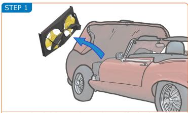
Disconnect the vehicle battery and remove the original fan shroud assembly according to the workshop manual. Remove the radiator side retaining bolts and keep in a safe place for re-installation. For this kit installation, the radiator can remain in-situ.
