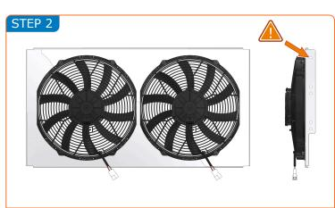
Lay the supplied shroud down on a workbench and align the fans as shown above. Note, the holes down the side of the shroud are offset toward the top of the shroud. Ensure the hole nearest the top of the side return is at the top.
