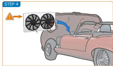
Carefully guide the fan and shroud assembly up to the rear of the radiator, ensure the fan cables are not snagged. Note the offset holes are closer to the top of the shroud.
