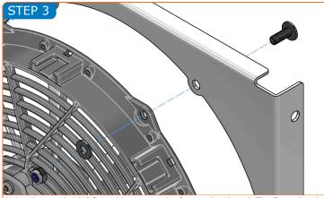
Using the suppled M6 fixing kits, secure the fans to the shroud. The flange head fixings are positioned through the shroud as shown - with the thread facing out. The fans fit flush against the fan shroud with a washer dropped on each thread before fully securing wuth a nyloc nut on each. Do not over-tighten.
