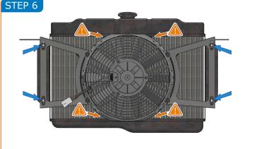
Loosen the 5/16" nyloc nuts and adjust the fan assembly to ensure the black plastic fan shrouds are both between the top and lower radiator tanks and are just touching the radiator core. Ensure the fans are free-spinning and that the assembly is not twisted. Check there is a uniform gap around the fan blades.
