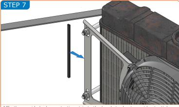
Affix the provided edge protection strip to the bracket edge to avoid potential damage to the wiring or oil cooler pipework
