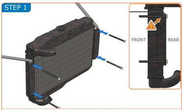
Disconnect the vehicle battery and drain the vehicle coolant system. Remove the top and bottom radiator fixing bolts that secure the radiator to the bulkhead. From the engine side, replace the bolts with the supplied 100mm long set screws. Note that the upper screws go through the diagonal braces.
