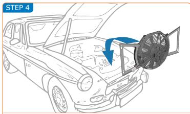
Position the fan assembly in the vehicle in the orientation shown in step 2 (shroud flats at the top). Make sure the fan assembly is pulled away from the radiator, just behind the bonnet catch panel to allow fitting of spacer tubes in step 5.
