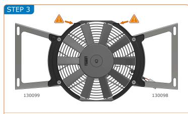
Flip over the assembly and ensure the brackets and black plastic fan shrouds are aligned as shown. Noting that the shrouds have a flat at the top. Fully tighten the M6 screws assembled in step 2, but do not overtighten.
