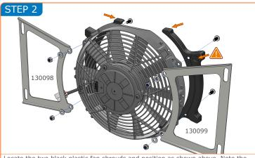
Locate the two black plastic fan shrouds and position as shown above. Note the dimple on the right hand shroud. From the rear, insert the four M6 screws through the fan shroud, fan body and side brackets. Place an M6 washer over each protruding screw thread before securing with an M6 nyloc.
