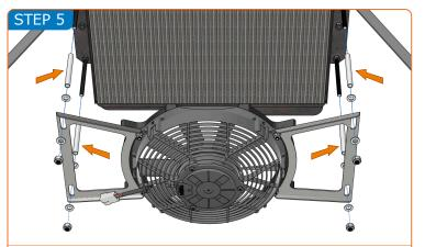
Slide the four spacers onto the screws from step 1. Use the longer spacers for the lower screws and the shorter ones for the top screws. Add an M8 washer to each screw, then slide the fan brackets over the threads. Place another M8 washer on top of each bracket and loosely tighten a 5/16" Nyloc nut
