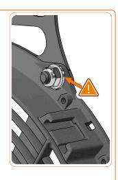
To assemble the fan kit, refer to the illustration above. You'll notice that both the upper and lower brackets are equipped with integral studs. Guide these studs through the corresponding fixing holes on the fan shroud. Once the studs protrude, place an M6 washer onto each, followed by an M6 nyloc nut, and tighten to secure the brackets firmly. Once the fan kit is fitted to the vehicle, ensure the fan blade is free-spinning and that the assembly is not distorted.
