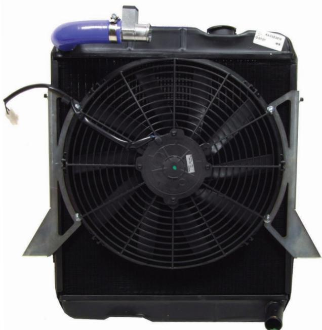
1. Disconnect +ve battery terminal, drain water system and remove the top and bottom hoses from the radiator. Remove the original fan and spacer from the water pump and use the pulley short bolt kit to re-fit the water pump pulley.
