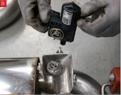
C) Rotate Scorpion valve so its in the same position as the O.E electronic valve motor.
