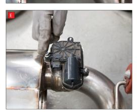
D) Once happy spring and Scorpion valve position are in line now fit the O.E electronic valve motor.
