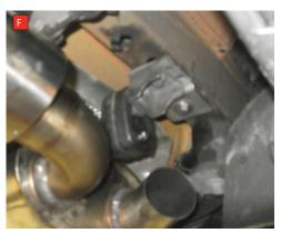
E) Using the 3 x 8mm O.E nuts secure in place. Once this is done now repeat on the other side.
