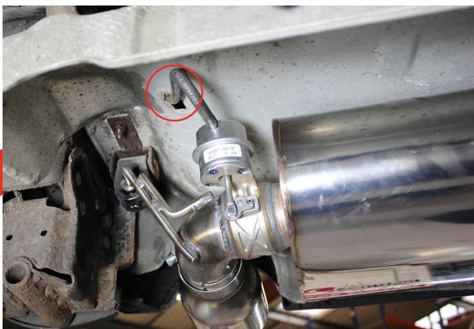
Once the Scorpion system is fitted re-route the vacuum valve hose back on itself, then through the hole in the heat shield as shown in the image, once re-routed connect the hose to the Scorpion valve.
