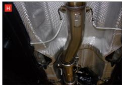
A) Prior to removing the original downpipe the heat shield needs to be removed. The black bracket on the heat shield is no longer required disconnect this by drilling out the two rivets circled in the picture.
