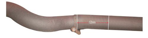
MEASURE FROM THE WELD ON ORIGINAL EXHAUST 120mm TOWARDS BACK OF CAR, MARK THE PIPE THEN CUT ORIGINAL PIPE, MAKING SURE THE PIPE WORK STAYS SQUARE.
