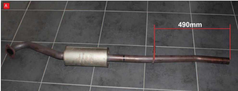
A) To fit the Scorpion rear silencer you will need to cut the O.E centre section. Carefully remove this and accurately measure 490mm from the bracket as shown in figure A and carefully cut the pipe work. Once cut clean and de-bur the cut end. Re-attach the centre section to the car and follow the line diagram on the previous page.
