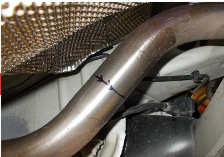
When fitting the rear silencer the original system requires cutting in a specific place. Cut the pipe directly between the two bends as marked in the picture.
