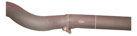
MEASURE FROM THE WELD ON ORIGINAL EXHAUST 120mm TOWARDS BACK OF CAR,
