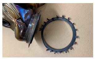
Remove the original gaskets from the original downpipe as they are required when fitting the Scorpion downpipe.
