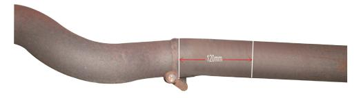
MEASURE FROM THE WELD ON ORIGINAL EXHAUST 120mm TOWARDS BACK OF CAR, MARK THE PIPE THEN CUT ORIGINAL PIPE, MAKING SURE THE PIPE WORK STAYS SQUARE.
