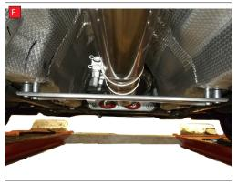
F) Using item 13 you will need to space out the bracer bar as shown. Use the O.E bolts.
