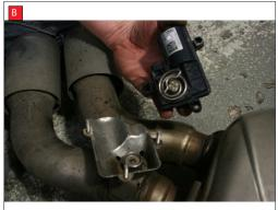
A) After you have removed O.E exhaust you will need to remove the two rear valve motors (Right hand side and left hand side). remove 6 x 8mm nuts from both sides (3 on each valve).
