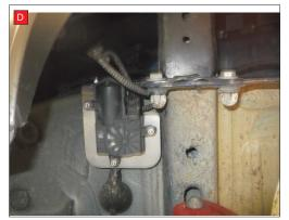
D) Using Items 9, 10 and 11 bolt the L/H O.E valve to item 7, then using item 12 bolt to the the car as shown in the photo. Item 7 will have engraved which hole the O.E stud needs to mount to.
