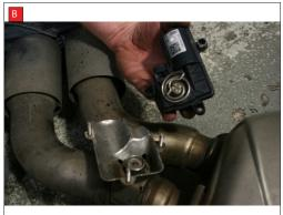
A) After you have removed O.E exhaust you will need to remove the two rear valve motors (Right hand side and left hand side). remove 6 x 8mm nuts from both sides (3 on each valve).
