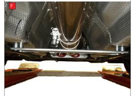
A) After you have removed O.E exhaust you will need to remove the two rear valve motors (Right hand side and left hand side). remove 6 x 8mm nuts from both sides (3 on each valve, keep safe as you will need them to bolt the electronic valve motors to Scorpion Exhaust).
