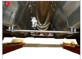
A) After you have removed O.E exhaust you will need to remove the two rear valve motors (Right hand side and left hand side). remove 6 x 8mm nuts from both sides (3 on each valve, keep safe as you will need them to bolt the electronic valve motors to Scorpion Exhaust).
