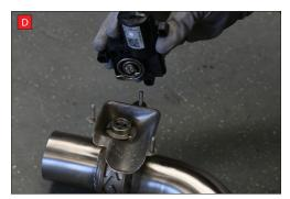
B) Lift up the motor. You will now be able to see the torsion spring (This must stay on the electronic valve motor to work with Scorpion Exhaust).
