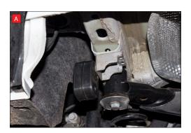
A) Both of the rear mounting points need rotating 180° when fitting the Scorpion exhaust.
