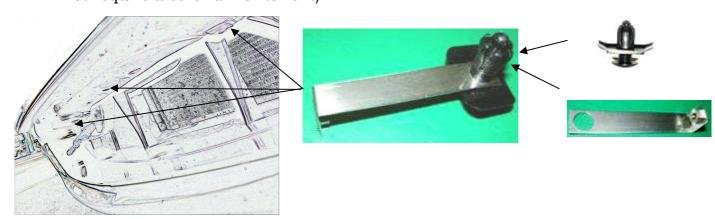
3. Using the Mesh grille as a guide for position, prize the lower bumper skin away from the lower bumper reinforcement and insert the 3 lower fixing clips.
