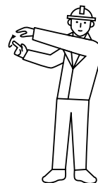
MOVE SLOWLY. Use one hand to give any motion signal and place other hand motionless in front of hand giving motion signal. (Hoist slowly shown as example.)
