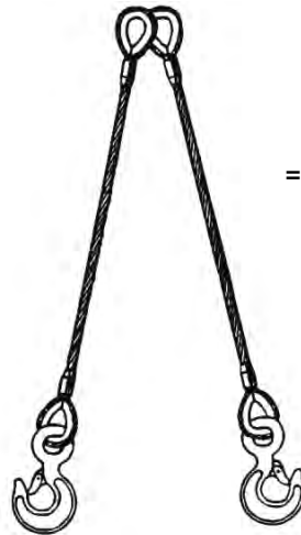
Figure 15.18 Two single legs in straight lift
