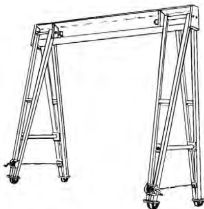
Figure 12.11 Self erecting gantry
