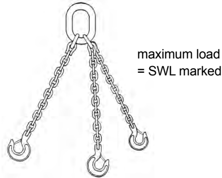
Figure 14.26 Three leg sling in straight lift
